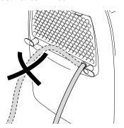
Remove the hose if you want to collect the condensate in the condensation tank again. Allow the hose to dry prior to storage.
