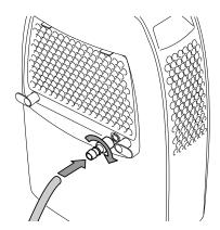
8. Guide the other hose end to a suitable drain or sufficiently dimensioned collection container. Please note that the hose must not be kinked.
