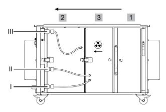
Then connect the two sensor hoses on the sensor hose side in accordance with the selected configuration:
