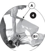
5. Hold on to the opening flap (A) and at the same time push the "short" fixation disc (B1) upwards while standing up.
